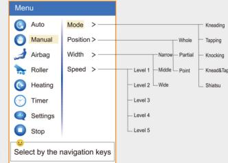
Manual massage:On Main interface, press "Manual" to convert to Manual Interface, There are 4 manual massage programs for selection: mode, massage position, width, speed.then
